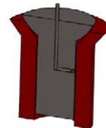
9. Check the coaxiality of a conic seat and a bore
