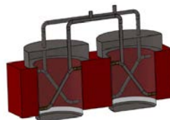
11. Checking the parallelism of two bores
